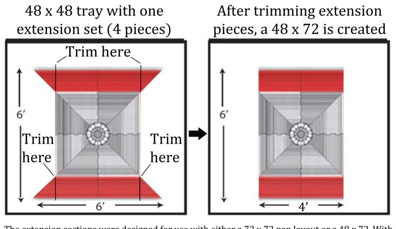
The extension sections were designed for use with either a  $72 \times 72$  pan layout or a  $48 \times 72$ . With the  $48 \times 72$  layout, you must trim the triangular section from each of the four extension pieces as shown. Any fine-toothed hand or power saw will easily accomplish this task.
