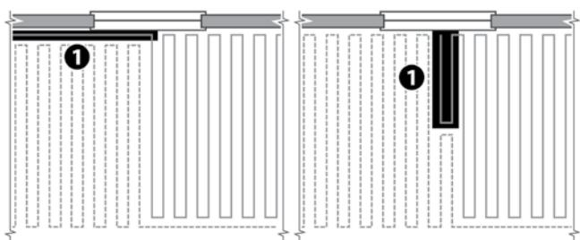
1. End the installation of the first cable by the wall, so that the second cable nestles in easily.
