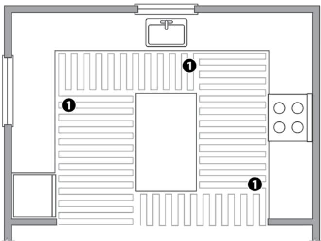
1. Change directions so the cable can be installed to the closest spacing allowed from walls and fixed furniture.
