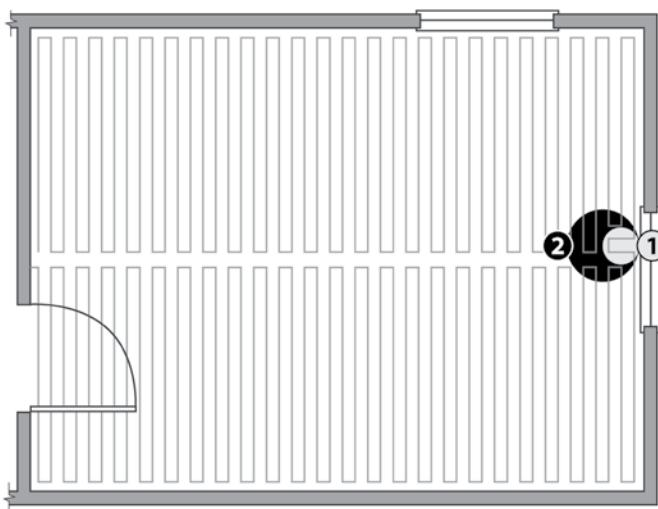
1. Do a small detour to break up the cable run.
